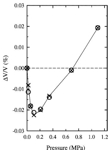
**Figure 7.** Dependence of the deformation of carbide-derived activated carbon upon the argon adsorption at 243 K measured by the dilatometric method<sup>1,35</sup> (open circles) and computed from the proposed method (crosses).
