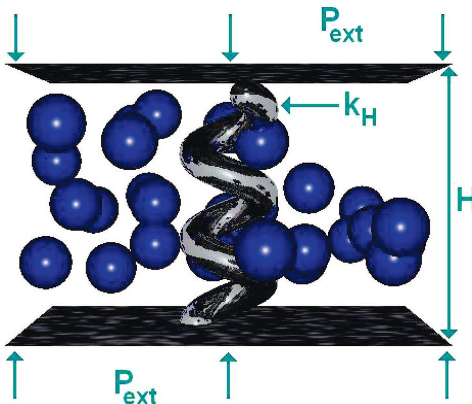
**Figure 1.** Slit-shaped carbon pore with adsorbed argon molecules:  $H$ , pore width;  $P_{\text{ext}}$ , external pressure;  $k_H$ , elastic element characterized by local elastic modulus.
